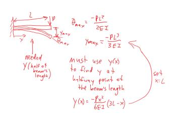
$$\left(\frac{B_{\gamma}L^{3}}{3EI} - \frac{5PL^{3}}{6EI} = 0\right) \times \frac{6EI}{L^{3}}$$
