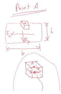
At A, Fy causes NO shear stress
